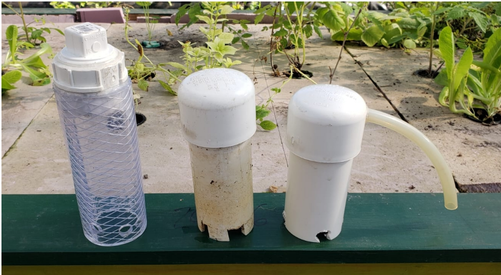
Figure 4.2 The three bells utilized in trials; (1) on the left there's the clear flexible tube with glued twisting cap, (2) on the center the PVC tube and cap, (3) at the right PVC tube and cap with a snorkel incorporated
